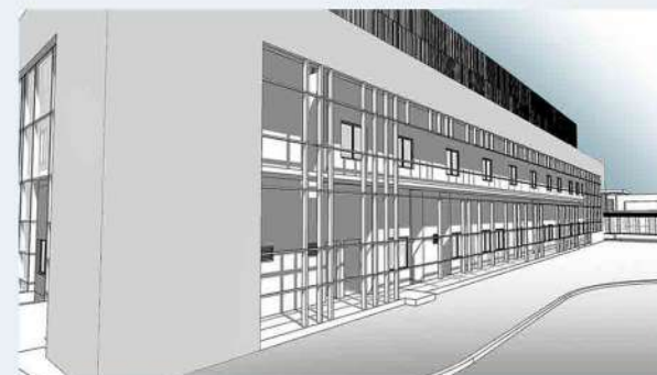
2. Addition of vertical and horizontal MS mullions as support members.
