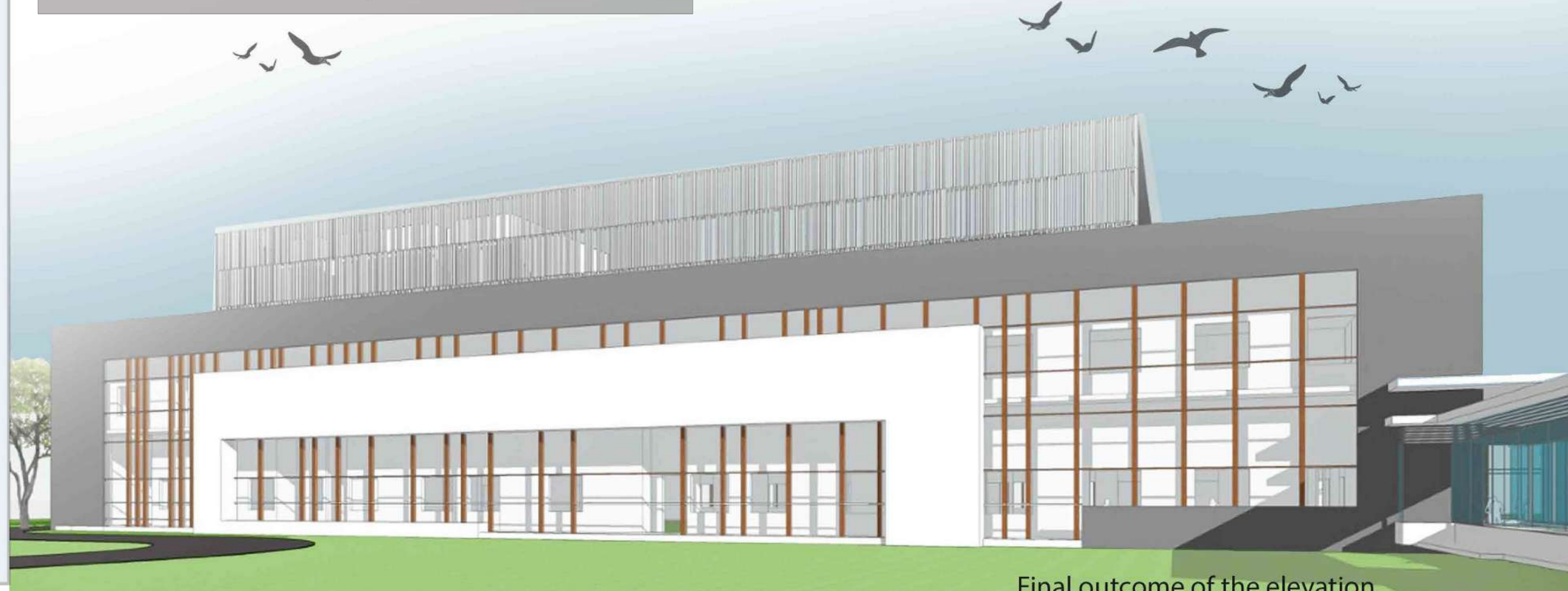
3. Placing tensile fabric as elevation element regulating the climatic characteristics
