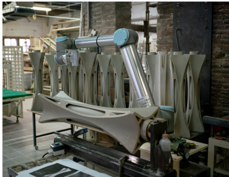
Robotic Arm Cutting Prototypes with Ceramica Cumella
