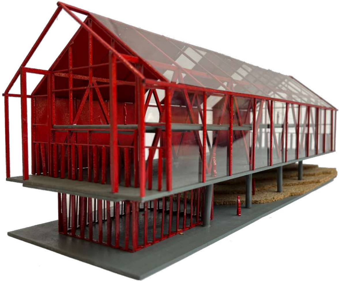
PART MODEL: FAB LAB EXTENSION AT 1:100 SCALE MATERIALS USED: MDF, ACRYLIC & CORK
