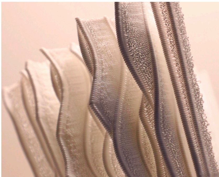
Additively Manufactured Textile. Source: Collateral Computation (Patel, 2023)
